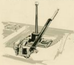
Rear end of unit power plant—silent Jeffery gear shift and emergency brake on propeller shaft.
