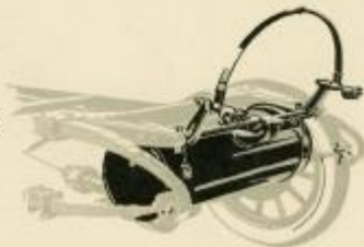
Rear view of chassis—extra size carrier, cylindrical gasoline tank and extra length rear springs
