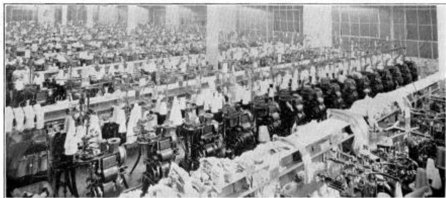
A SECTION OF CIRCULAR HOSIERY MACHINES
