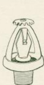
GRINNEL SPRINKLER, CLOSED.
