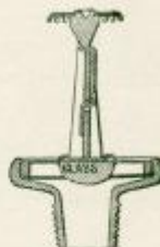
GRINNEL SPRINKLER, SECTIONAL.
