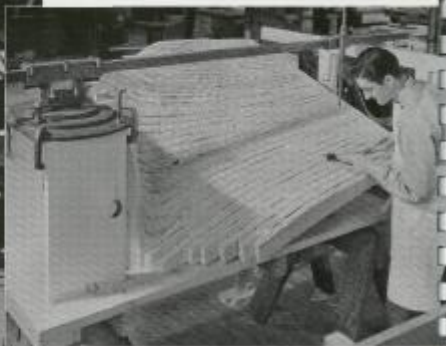
(Above) First step in making the pattern of a propeller blank.
