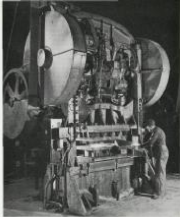
(Above): Drawing a Sch-Zero compressor component part on large press.
