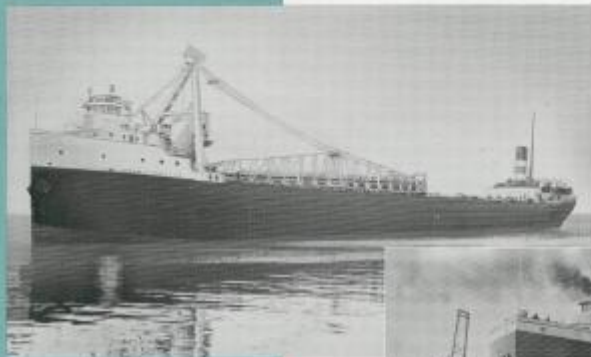
(Above) The steamer ADAM E. CORNELIUS of Island A. Greenlee, Buffalo, N. Y., was converted to a self-loader in 1930.
