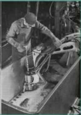
Spot welding back on Sub-Zero inner jacket.
