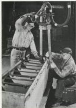
Spot welding head frames inner jacket.
