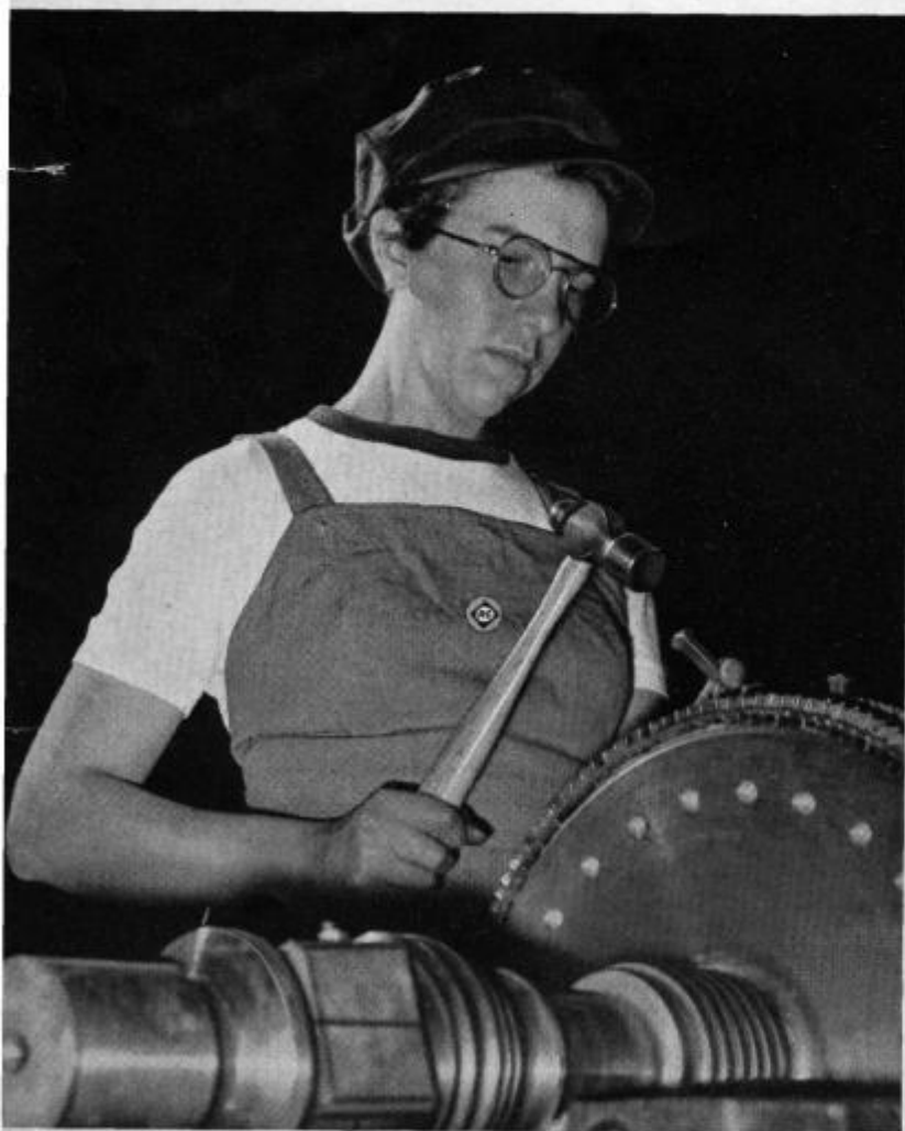
Antoinette Schmitz, West Allis, recruited from the N. Y. A. industrial training center, sets blades in small naval steam turbines.
