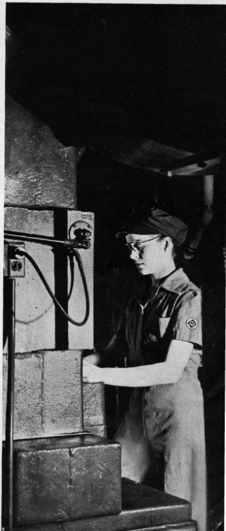
Punching out small turbine parts for use on battleships and in vital power stations is the job Martha Kalember, West Allis, is doing.
