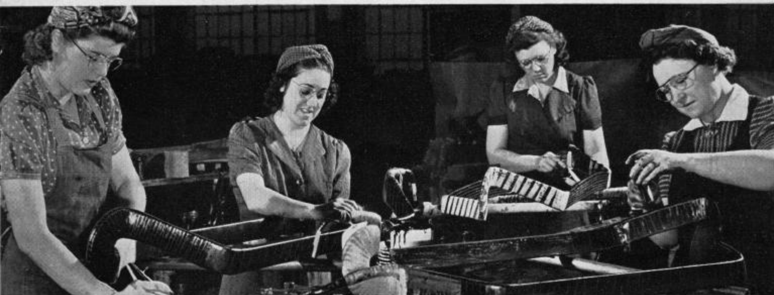
Ann Zacek, Ann Calabrese, Vera Stahl, and Marie Bucholtz insulate a stator coil for a basic magnesium plant—a job that calls for precision.
