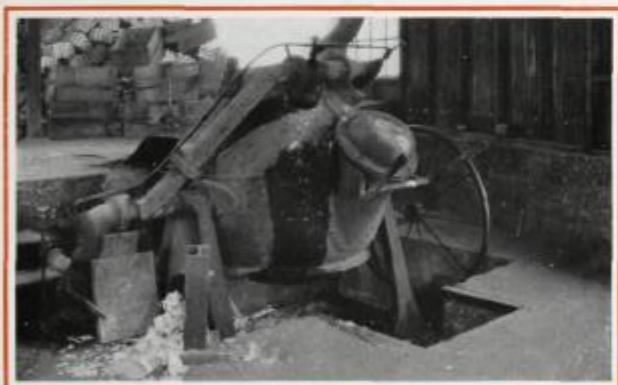
4 Heating furnace in which ingots are melted and all dross skimmed off. Only the pure metal is used in making Mirro.
