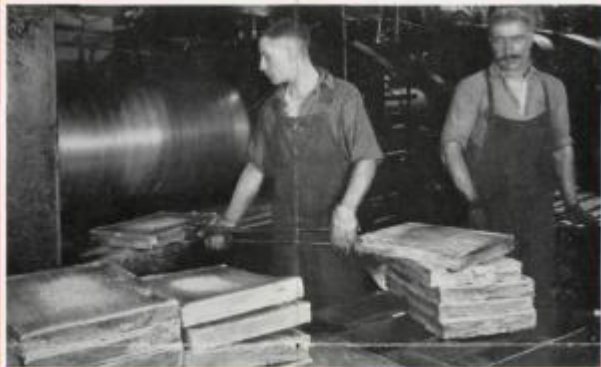
7 Slabs are rolled and cross-rolled under eight tons pressure reducing them to plates one-quarter inch thick.
