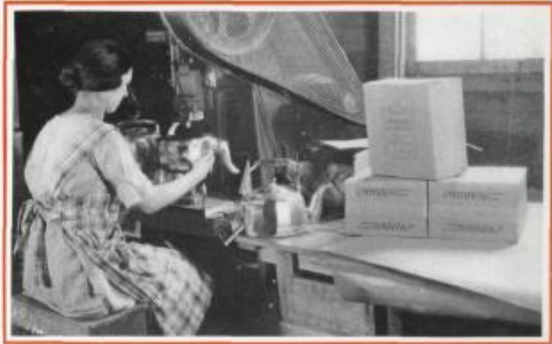
16 After buffing and polishing, the Mirro trade mark is put on so you can always identify Mirro.
