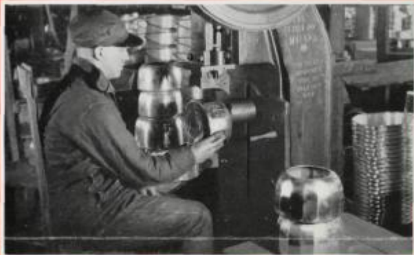
13 Stamping the Colonial pattern. The angles add strength to Mirro Colonial designs.
