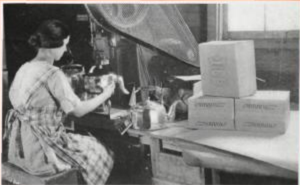
16 After buffing and polishing, the Mirro trade mark is put on so you can always identify Mirro.
