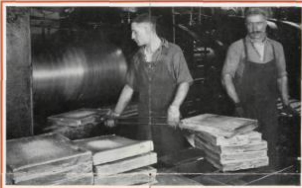
7 Slabs are rolled and cross-rolled under eight tons pressure reducing them to plates one-quarter inch thick.
