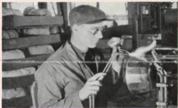
15 Welding on the spout. Mirro utensils are perfectly smooth, both inside and out.
