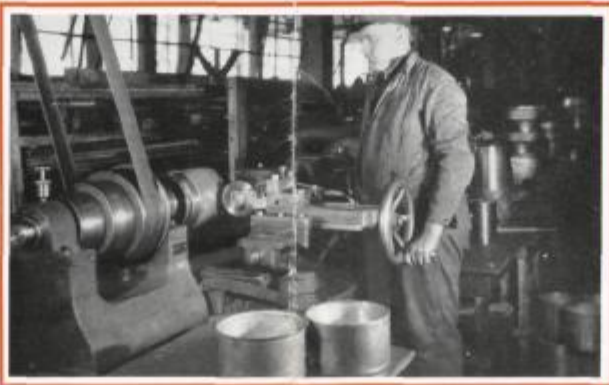
10 Rolling and ironing. This process closes the pores of the metal and irons out the wrinkles.
