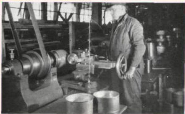
10 Rolling and ironing. This process closes the pores of the metal and irons out the wrinkles.
