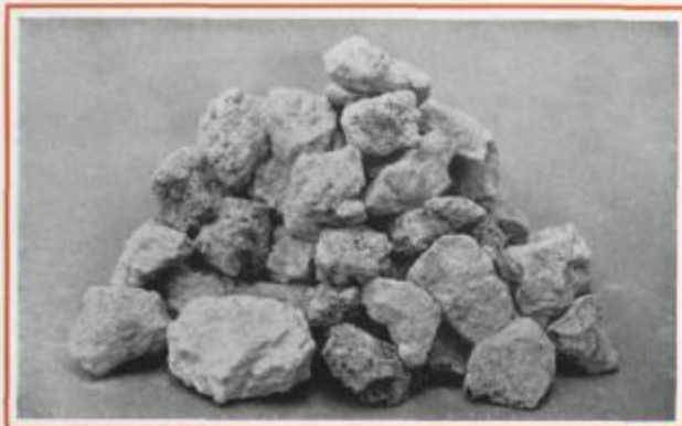
1 BAUXITE—the clay which is the basis of all aluminum.
