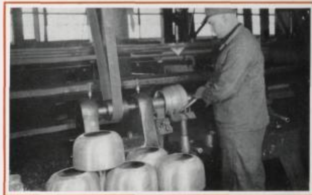
11 Spinning—the process which gives Mirro utensils their graceful shape.
