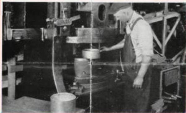
9 Cold stamping and drawing. Some Mirro utensils are given twelve draws to insure uniformity of thickness.
