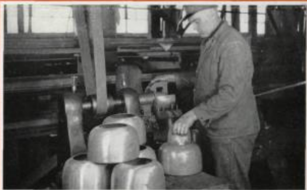
12 Removing split chucks from utensils after the spinning is done.
