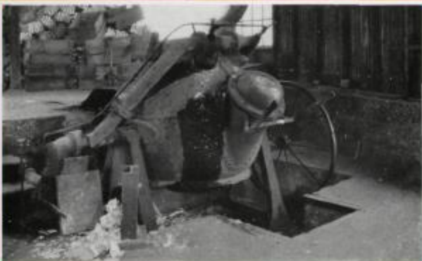
4 Heating furnace in which ingots are melted and all dross skimmed off. Only the pure metal is used in making Mirro.
