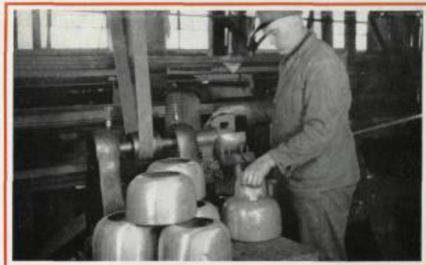
12 Removing split chucks from utensils after the spinning is done.
