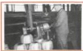
11 Spinning —the process which gives Mirro utensils their graceful shape.
