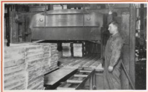
6 Slabs are then heated to high temperature preparatory to breaking down into plates.
