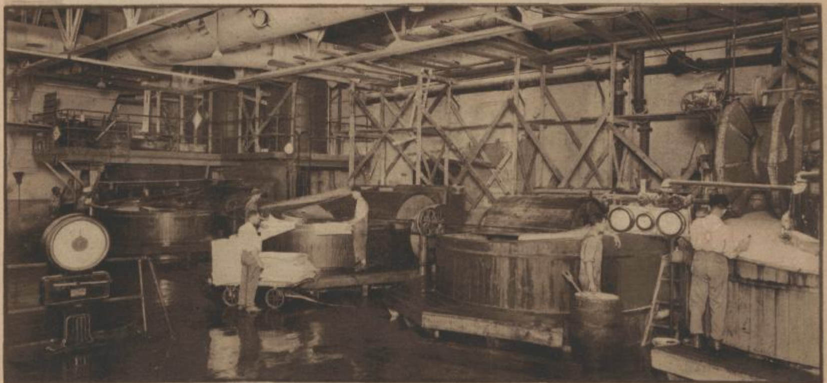
The last word in beating engines is the Niagara Beater , doing the work of four beaters of twenty-five years ago. The distinctive feature of the Niagara Beater is the sloping bottom which hastens the flow of the stock.
